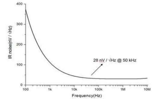
Figure 8. Noise simulation result of pre-amplifier
