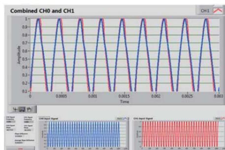
Figure 30. Phase difference measurement result between two channel
