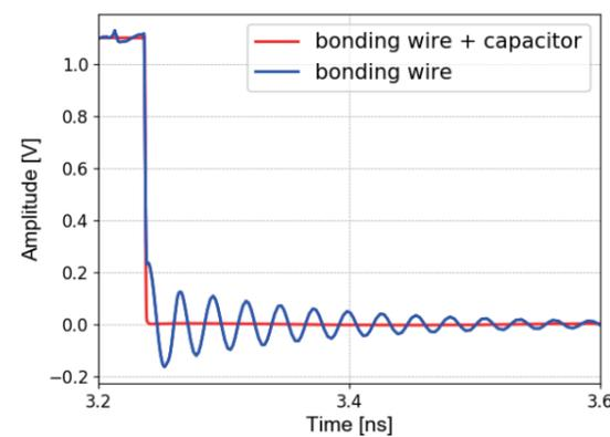
Fig.15. Ringing effect of bonding wire
