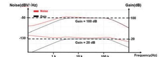
Figure 27. Noise simulation result with minimum gain and maximum gain
