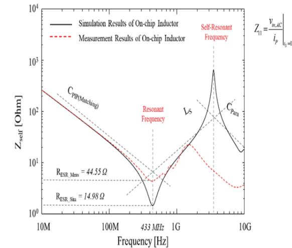
Fig. 13. The self-impedance  $Z_{self}$  measurement result of the fabricated on-chip inductor pattern.
