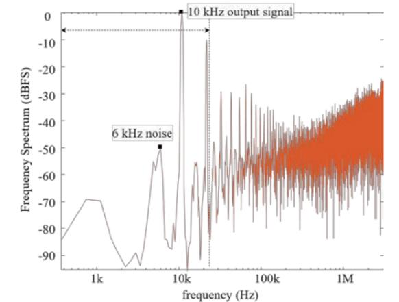
Fig. 8. Simulated frequency spectrum of the designed sigma delta modulator with ground noise
