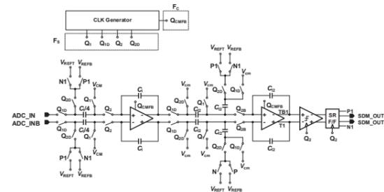
Figure 14. schematic of the designed Sigma-Delta Modulator (SDM)
