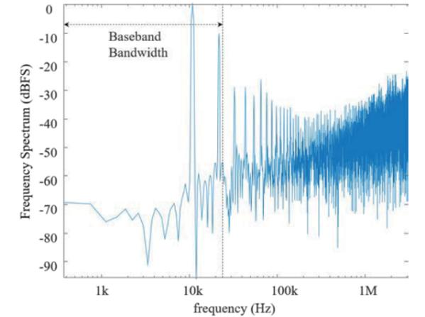
Fig. 7. Simulated frequency spectrum of the designed sigma delta modulator
