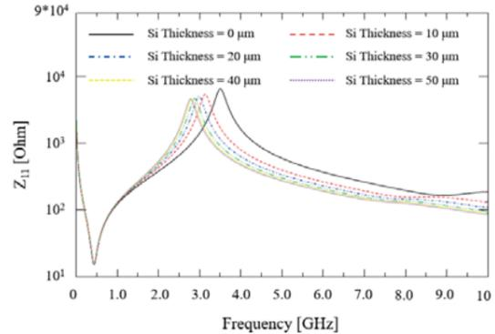
Fig. 8. Changes in the Self-impedance of the on-chip inductor with the variation of the Si substrate thickness.
