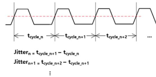
Fig.16. Concept of cycle-cycle jitter
