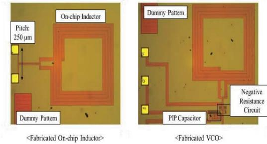
Fig. 11. Fabricated on-chip inductor and voltage controlled oscillator using SK Hynix 0.35  $\mu$ m process.
