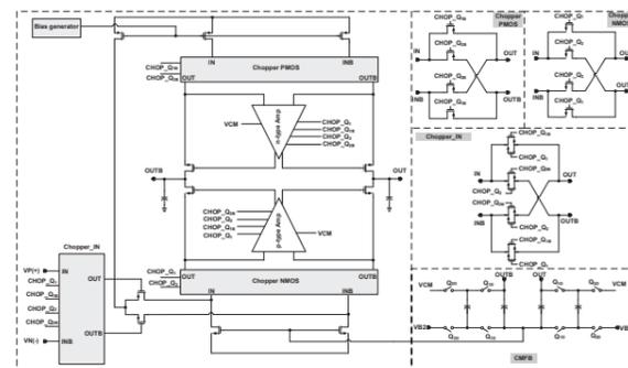
Figure 15. Schematic of OP-Amp in the proposed SDM
