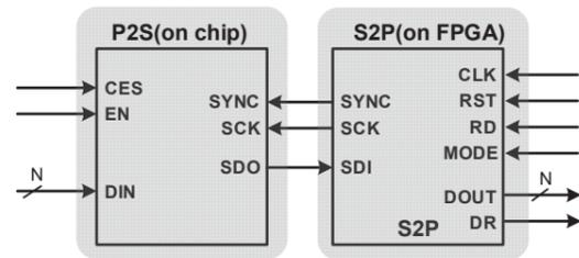
Figure 21. P2S and S2P block diagram
