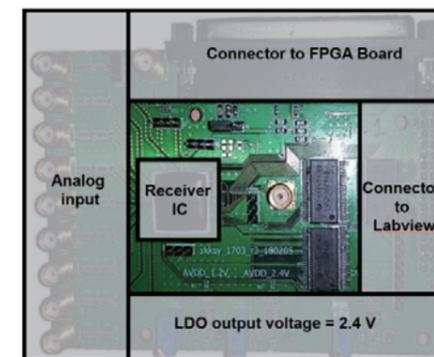
Figure 25. Evaluation board for the receiver IC
