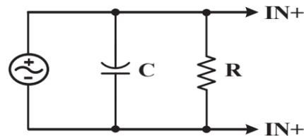
Figure 2. Equivalent circuit of sensor on the input
