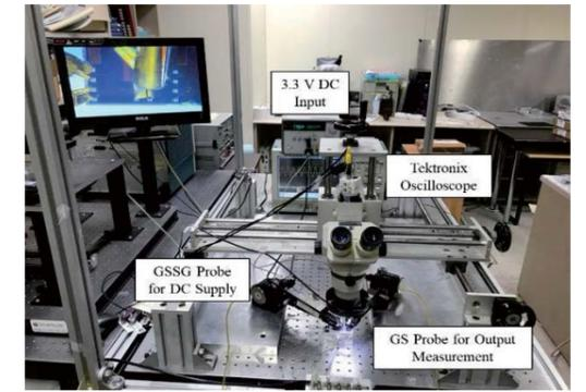
Fig. 14. The measurement setup of the fabricated voltage controlled oscillator (VCO) using the DC supply and oscilloscope.
