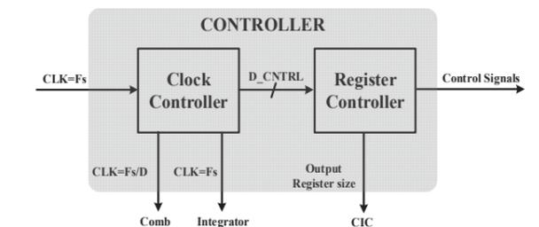
Figure 20. Proposed controller for configurable CIC filter
