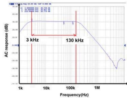
Figure 28. AC response of the band pass filter
