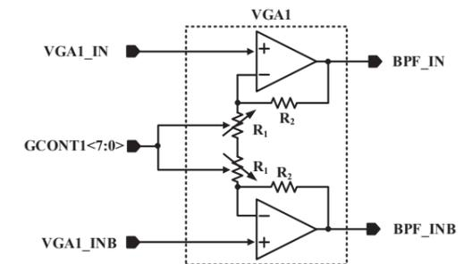
Figure 9. Schematic of VGA1
