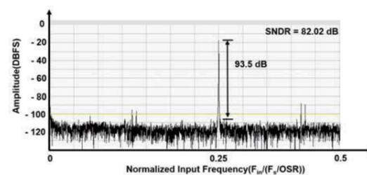
Figure 29. PSD measurement result of the proposed receiver with sinuswave input
