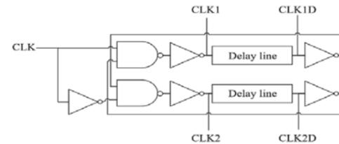
Fig. 3. Block diagram of the designed clock generator
