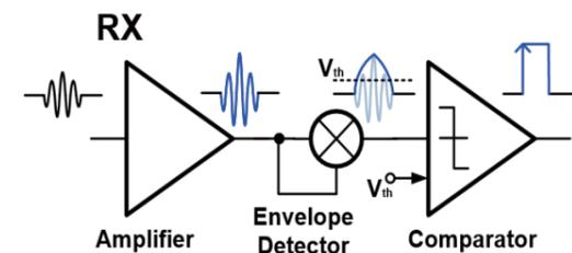
Fig.2. Analog front end receiver diagram
