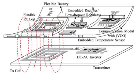
Fig. 1. Proposed wireless power transfer (WPT) scheme using the embedded flexible packages. Power will be delivered through the flexible coils using magnetic field resonance. The rectifier and regulator chips were embedded in the flexible PCB to rectify and regulate the received AC power. Finally, the regulated power will be delivered to the embedded VCO.
