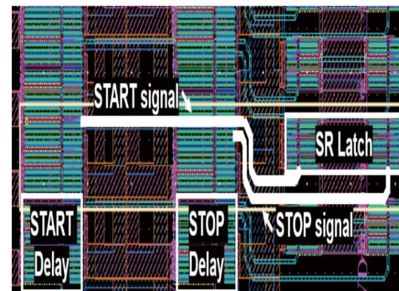
Fig.9 Asymmetry and non-uniform start and stop signal lines
