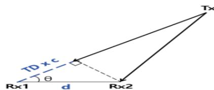
Fig.3. Principle of bearing angle measurement
