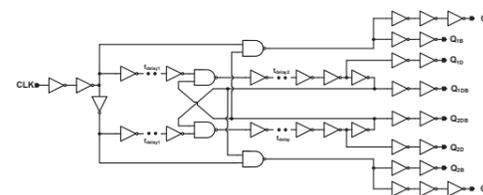
Figure 16. Structure of the non-overlap two-phase clock generator
