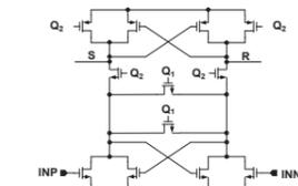
Figure 18. Structure of the comparator
