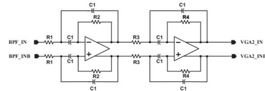
Figure 11. Schematic of Band-Pass Filter (BPF)
