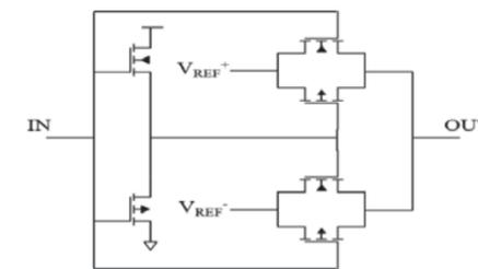
Fig. 6. Schematics of the designed 1-bit DAC.
