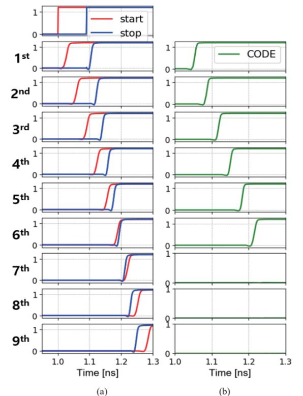
Fig.5. TDC timing simulation (a) START and STOP signal, (b) Thermometer code
