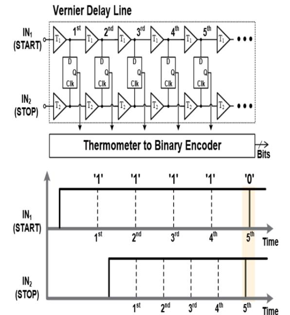
Fig.4 TDC block and timing diagram
