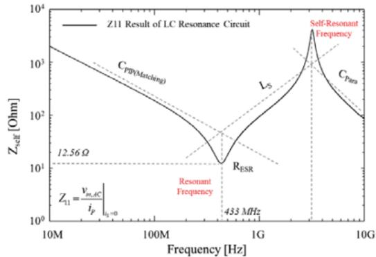
Fig. 7. Self-impedance ( $Z_{self}$ ) 3D EM simulation results of on-chip inductor. We optimize the on-chip inductor to achieve the higher Q-factor at the resonance frequency.
