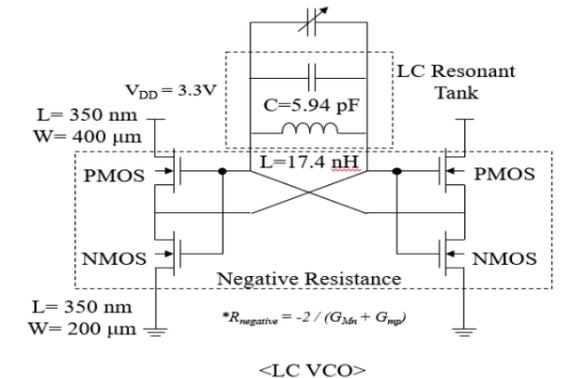
Fig. 6. Designed the LC -G<sub>M</sub> voltage controlled oscillator (VCO) circuit
