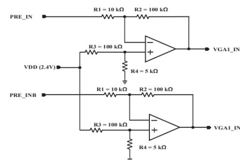
Figure 5. Schematic of pre-amplifier
