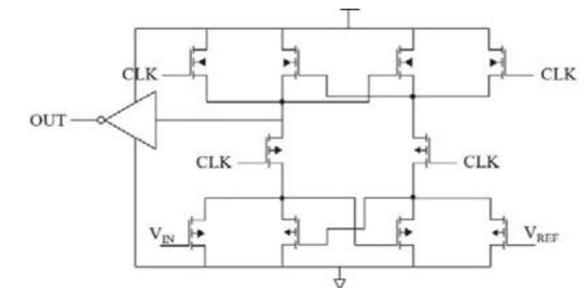
Fig. 5. Schematics of the designed latched comparator.
