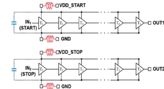
Fig.14. Schematic model with bonding wire inductance
