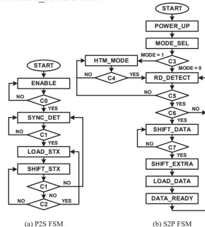
Figure 22. Serial interface FSM diagram
