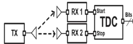
Fig.1. Bearing angle measurement system diagram
