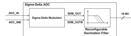
Figure 12. Simplified block diagram of the proposed SD ADC
