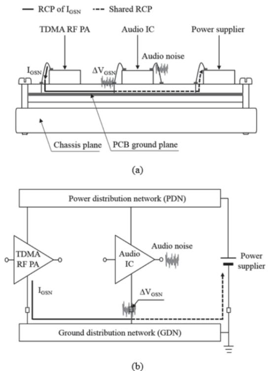
Fig. 1. Ground noise coupling mechanism between an audio IC and a TDMA PA in a smartphone. (a) Conceptual diagram (b) Block diagram.
