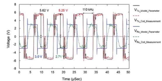
Fig. 4. Comparison between the time-domain voltage waveform simulation and measurement results.
