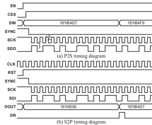
Figure 23. Serial interface timing diagram
