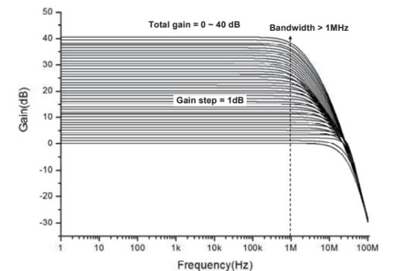
Figure 10. AC simulation result of VGA1
