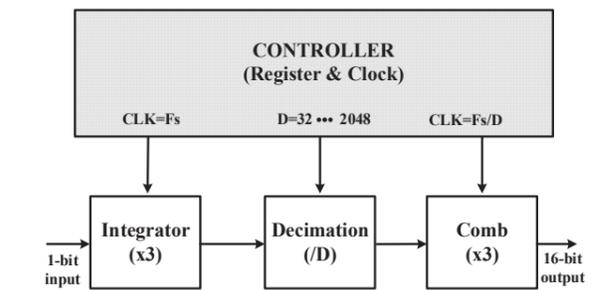
Figure 19. Proposed block diagram of the decimation filter
