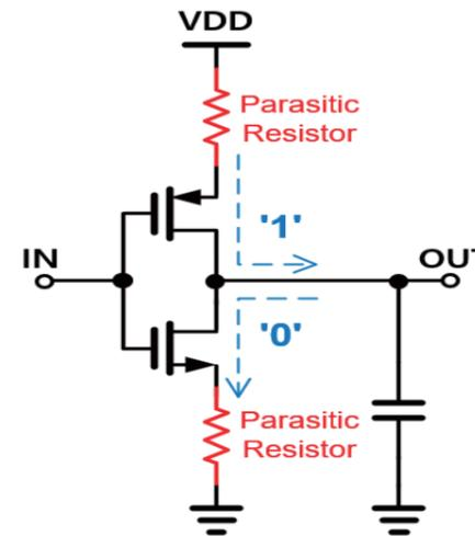
Fig.10. RC delay caused by parasitic resistance
