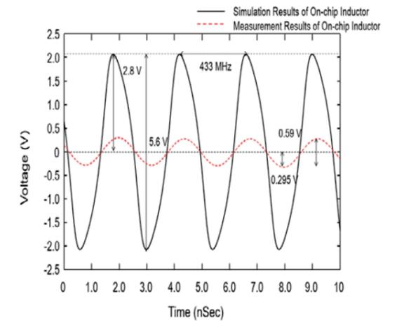
Fig. 15. The voltage waveform measurement result of the fabricated VCO using the Tektronix oscilloscope.
