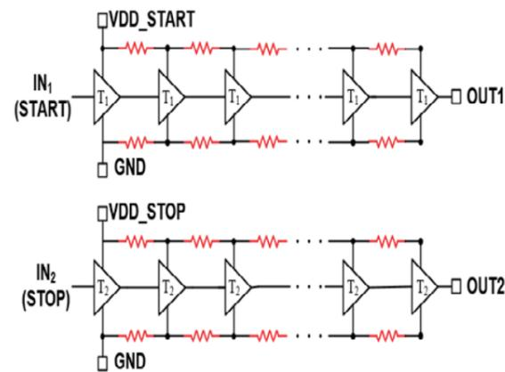
Fig.12. Schematic model with parasitic resistance
