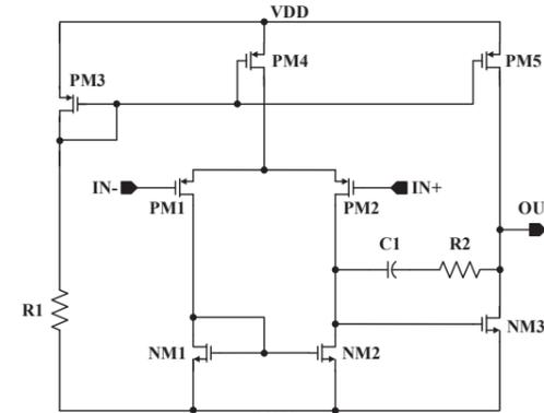
Figure 6. Schematic of OP-Amp in the pre-amplifier
