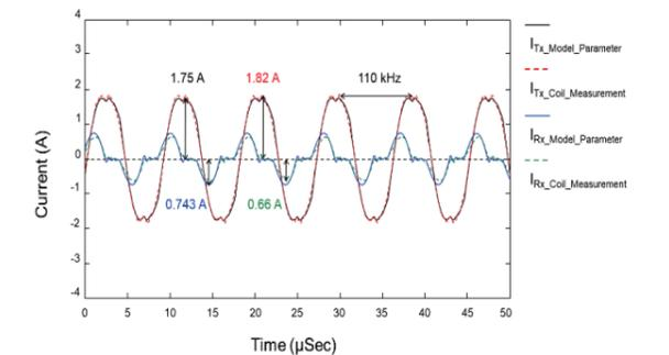
Fig. 5. Comparison between the time-domain current waveform simulation and measurement results.
