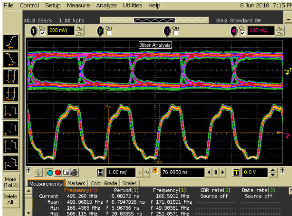
Fig. 21. Recovered Clock and Data(None jitter)
