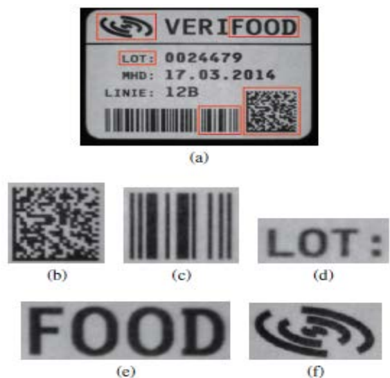
Fig. 12. (a) Reference image, (b)-(f) templates. Image courtesy of Baumer.
