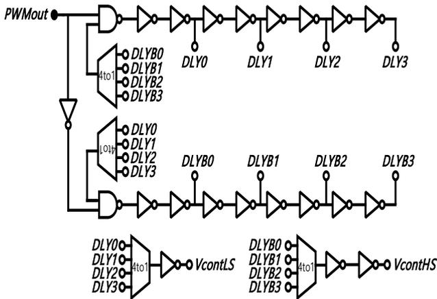
Fig. 6 Structure of dead-time generator
