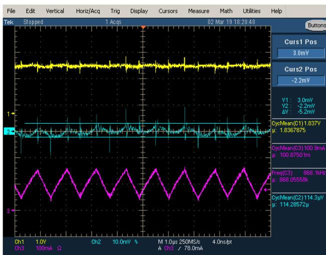
Fig. 10 Measurement result of 100 mA constant load condition
