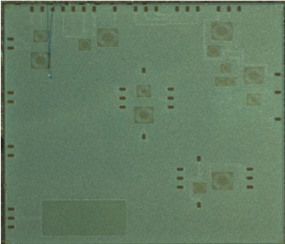
Fig. 13. The microphotograph of fabricated full duplexer.
