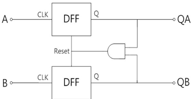
Fig. 5. Block diagram of the phase detector.
