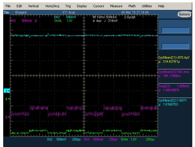
Fig. 12 Measurement result of a load transient condition from 100 mA to 300 mA
