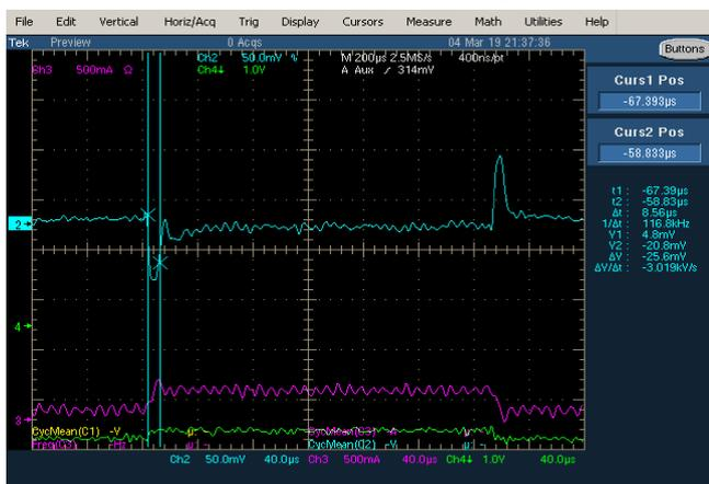
Fig. 14 Measurement result of output voltage undershoot
