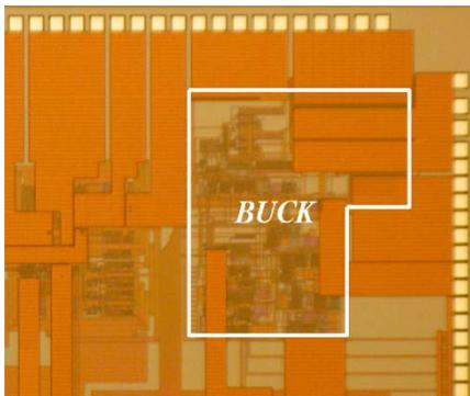
Fig. 5. The photograph of the proposed DC-DC buck
