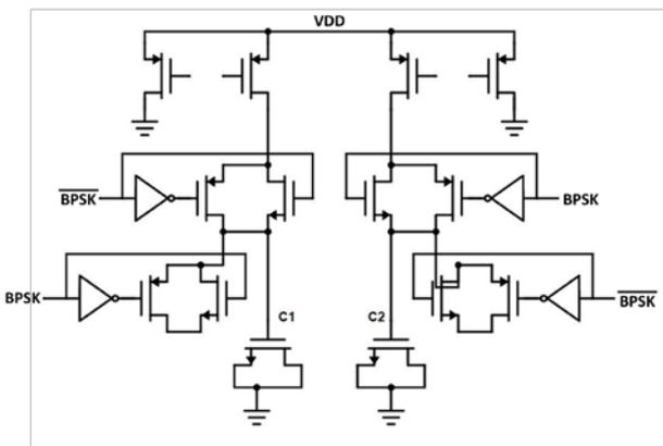
Fig. 6. Circuit schematic of Pulse-width measurement
