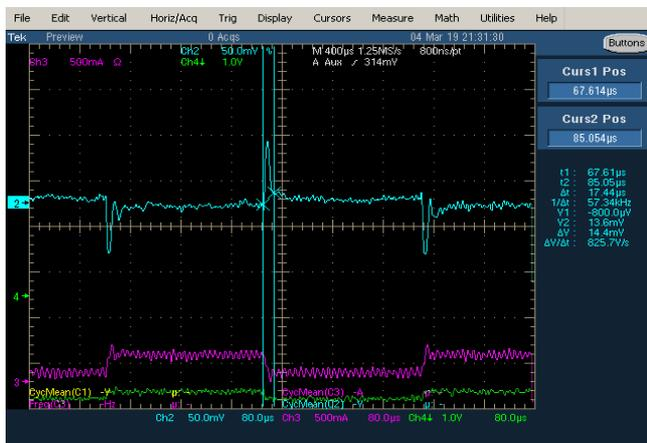
Fig. 13 Measurement result of output voltage overshoot
