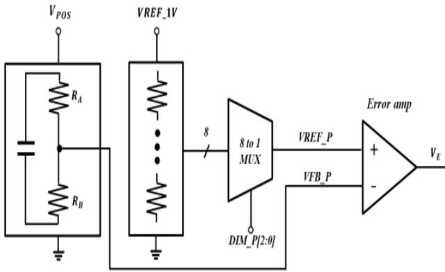
Fig. 4. Variable output voltage circuit for  $V_{Pos}$ .
