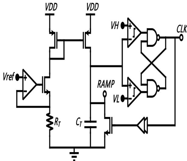
Fig. 4 Structure of ramp & clock generator
