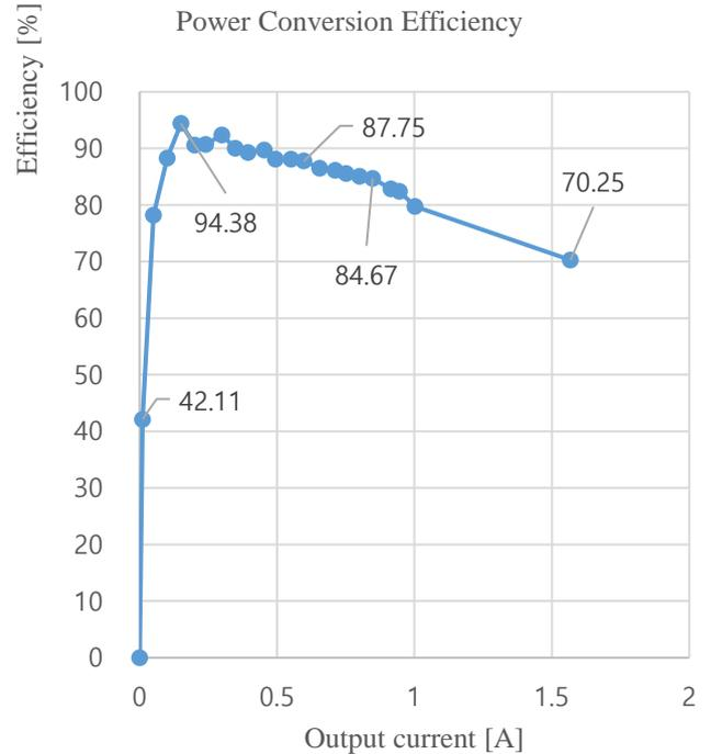
Fig. 11 Plot of PCE versus output current
