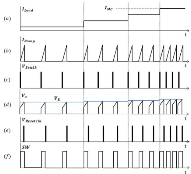
Fig. 3. Waveform of SPWM method (a) Load current  $I_{MC}$ , (b) Ramp current  $I_{Ramp}$ , (c) Set clock signal  $V_{setclk}$ , (d) Current sensing voltage  $V_C$  and error amplifier voltage  $V_E$ , (e) Reset clock signal  $V_{resetclk}$ , (f) Switching pulse SW.
