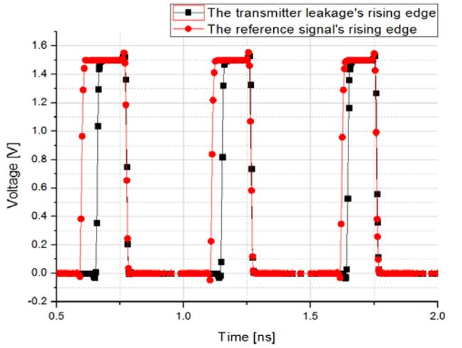
Fig. 6. Input and output voltages of the phase detector.
