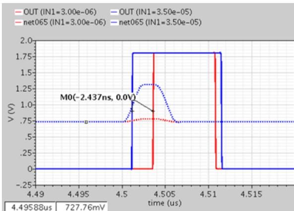
Fig. 11. Transient simulation result for the comparator according to the amplitude of the input voltage pulse.
