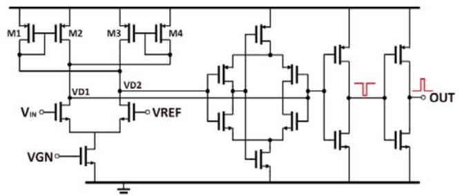
Fig. 9. Comparator schematic.
