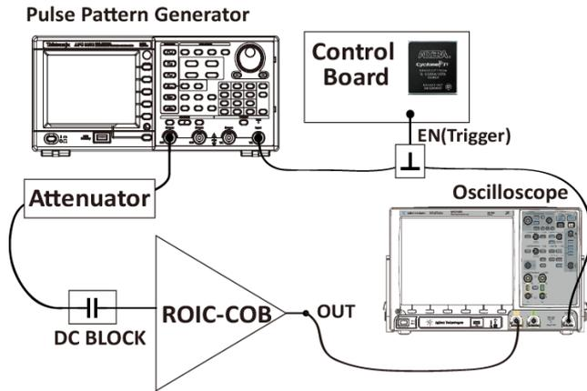
Fig. 5. Setup for fabricated chip test.
