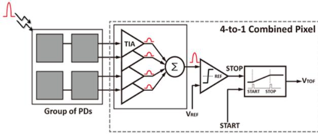
Fig. 2. 4-to-1 combined pixel architecture.
