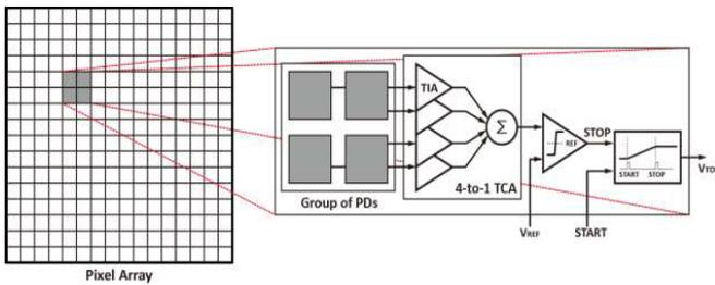
Fig. 3. Architecture of 8×8 pixel array with 4-to-1 combined pixels.
