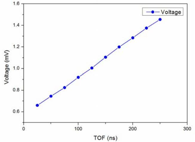
Fig. 18. Measurement result for T2V according to TOF from 8 × 8 array
