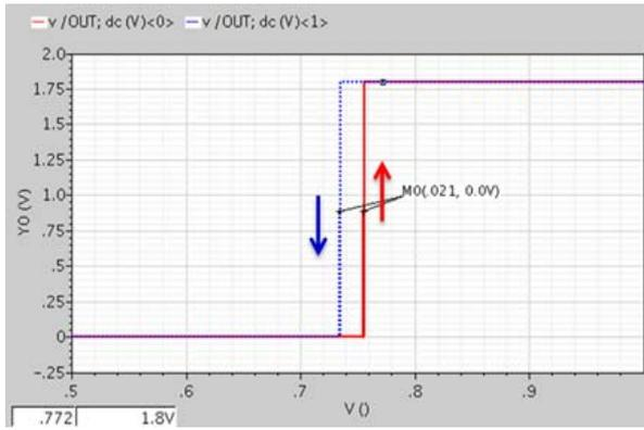
Fig. 10. Hysteresis simulation result for the comparator
