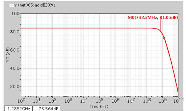
Fig. 7. AC simulation result for the 4-to-1 TCA
