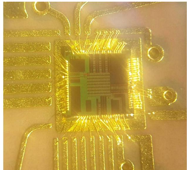
Fig. 15. Microphotograph of a designed 8 × 8 combined pixel array
