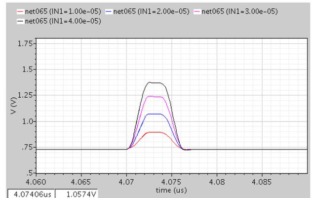
Fig. 8. Transient simulation result for the 4-to-1 TCA
