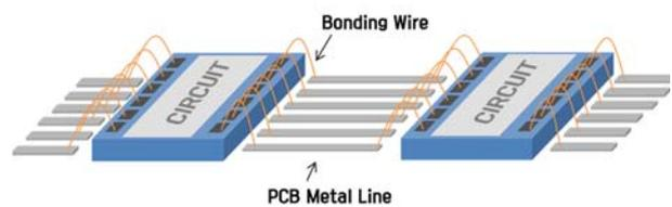
Fig. 1. Conceptual diagram of 2-D semiconductor technology
