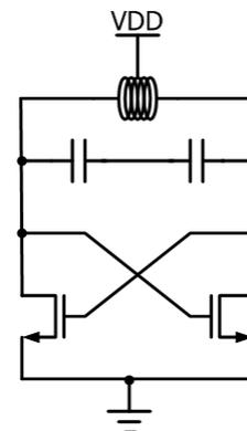
Fig. 2. Conventional cross-coupled oscillator structure
