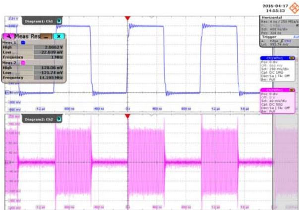
Fig. 12. Measured waveform of receiver coil
