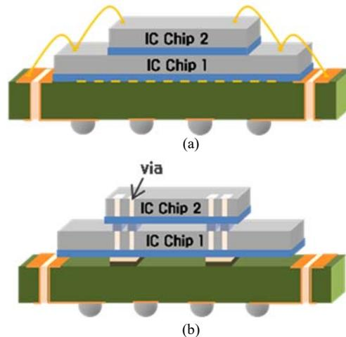
Fig. 2. 3-D IC (a)MCP technology (b)TSV technology
