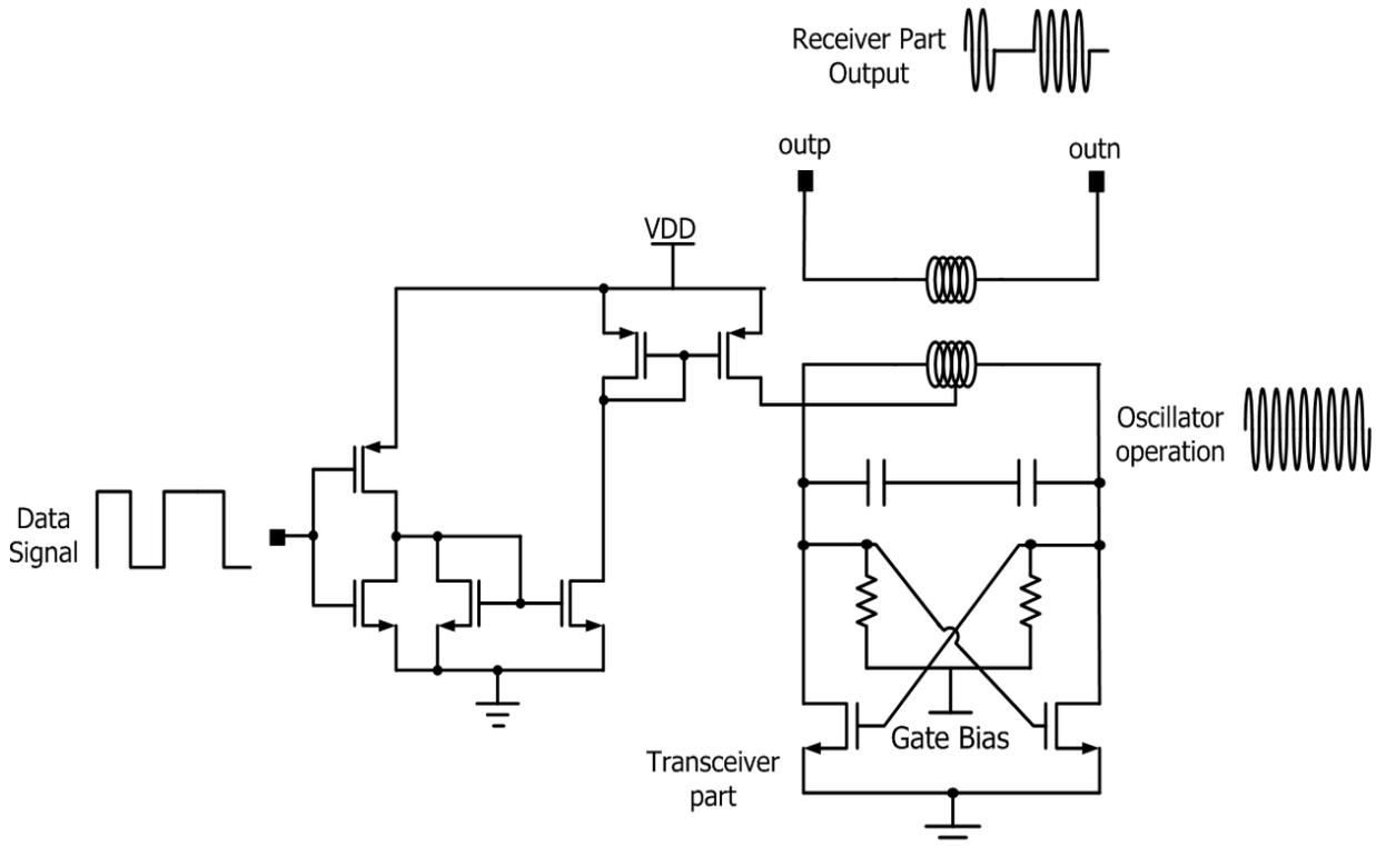
Fig. 5. Conventional wireless data transfer system for WCC circuit
