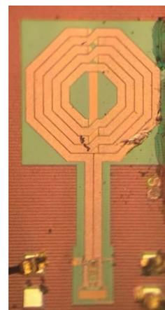
Fig. 11. Chip Photograph of the fabricated transmitter part
