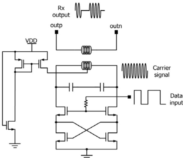
Fig. 6. Transmitter part for WCC circuit using cascode structure
