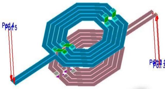
Fig. 7. EM simulation for Coil Characteristic
