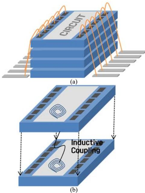
Fig. 3. (a) Conceptual diagram of wireless chip-to-chip communication (b) inductive coupling concept
