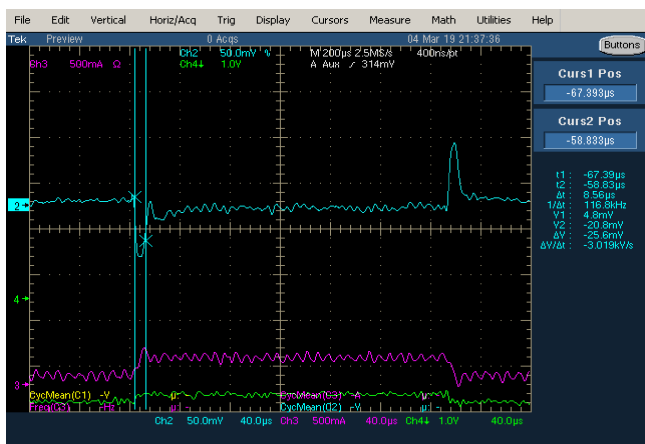
Fig. 14 Measurement result of output voltage undershoot
