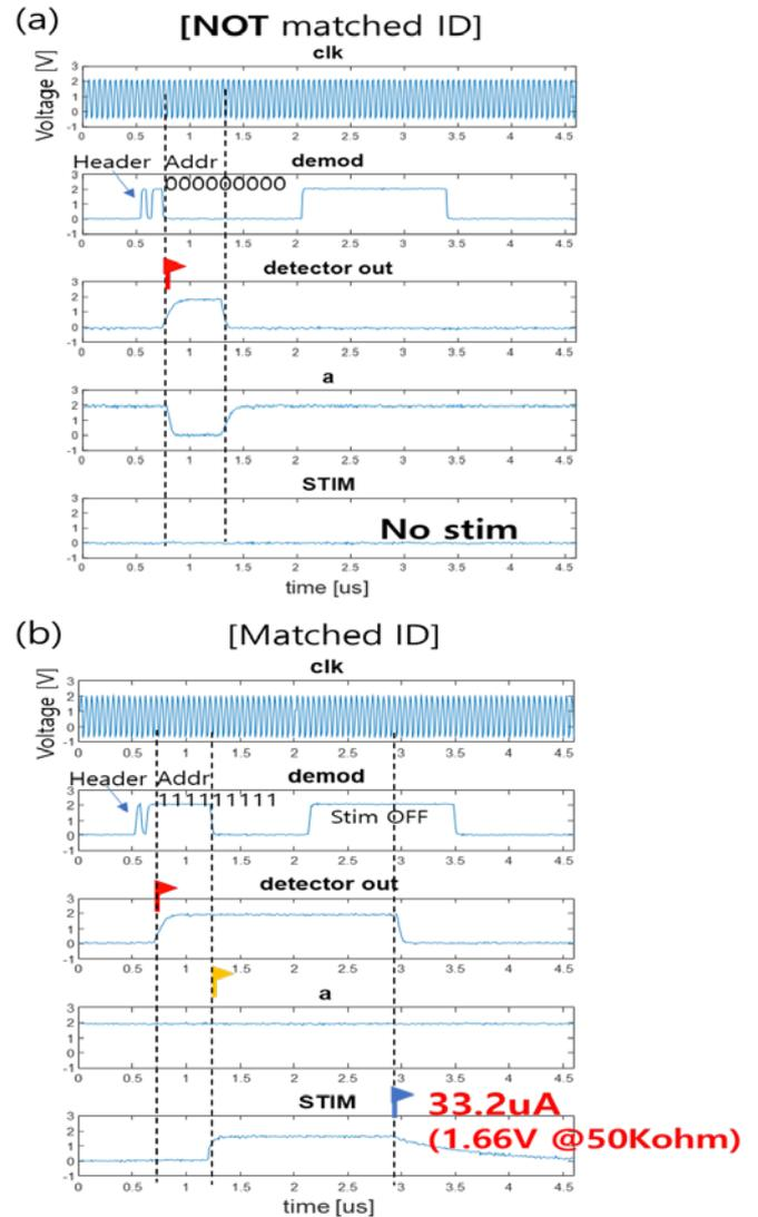
Fig. 9. Measured the digital block three outputs: the header detector 'detector\_out', address comparator 'a', and stimulation current 'STIM'; (a) when the addresses are not matched and (b) addresses are matched.
