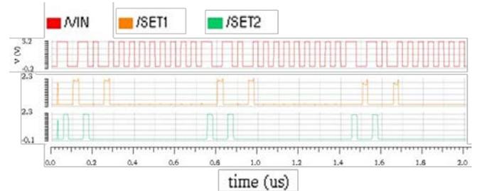
Fig. 7. Post-stimulated the rectangular pulsed voltage response of two Schmitt triggers (SET1, SET2) and BPSK input signal (VIN).
