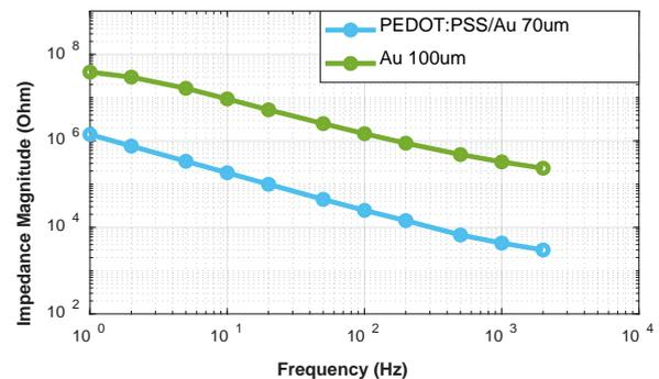
Fig. 10. Impedance spectra of Au and PEDOT: PSS/Au electrode
