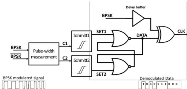
Fig. 5. Functional block diagram of analog circuitry
