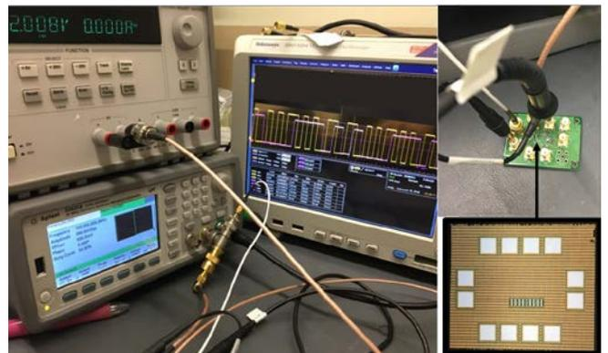
Fig. 4. Benchtop setup; The chip was wire-bonded on the PCB board and connected to a load resistance 50kohm.
