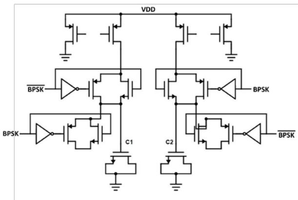
Fig. 6. Circuit schematic of Pulse-width measurement
