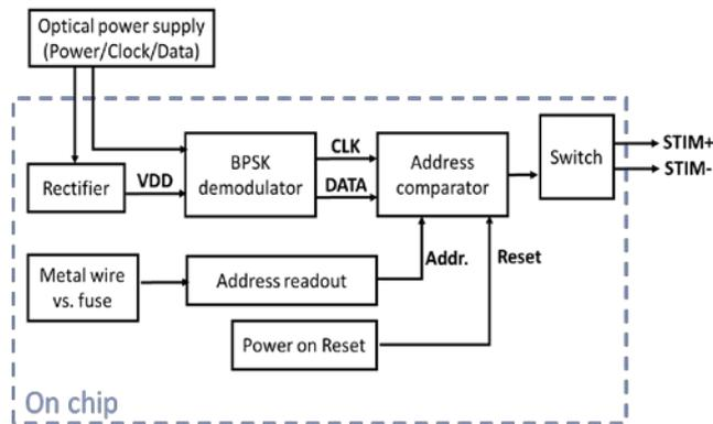
Fig. 3. Functional block diagram of neural implant system
