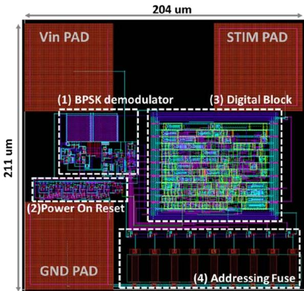
Fig. 11. Layout of the mixed mode chip in 0.18  $\mu$ m CMOS process
