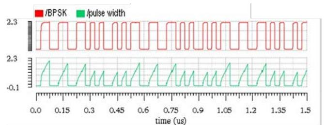
Fig. 6. Post-stimulated the voltage response across the capacitor in the pulse width measurement.
