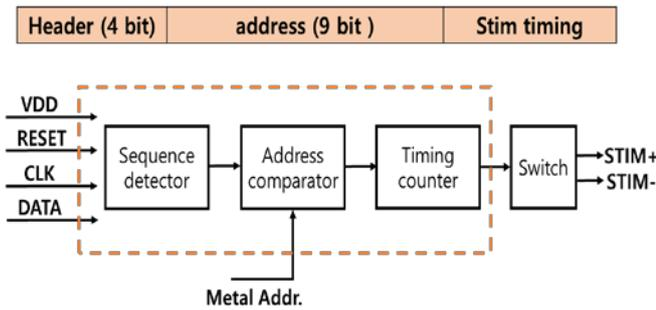
Fig. 8. A single data packet instructing stimulation current and the block diagram of the digital circuitry.
