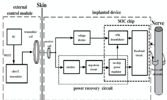
Fig. 2. Functional block diagram of wireless neural stimulating system [5]
