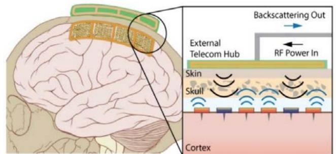
Fig. 1. The concept of a wireless neural implant('Neurograin') network.
