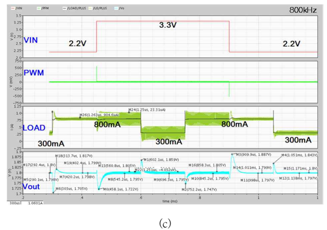
Fig. 13. Load line regulation of the buck converter: (a) For switching frequency of 3MHz, (b) For switching frequency of 1.2MHz, (c) For switching frequency of 800kHz
