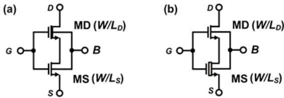
Fig. 3. n-channel self-cascode structure using optional devices. (a) ZVT (b) DGOX SC
