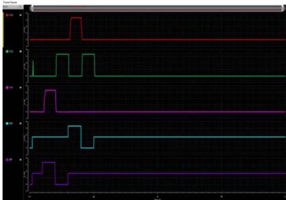
Fig. 14. Simulation waveform of bus failure detector
