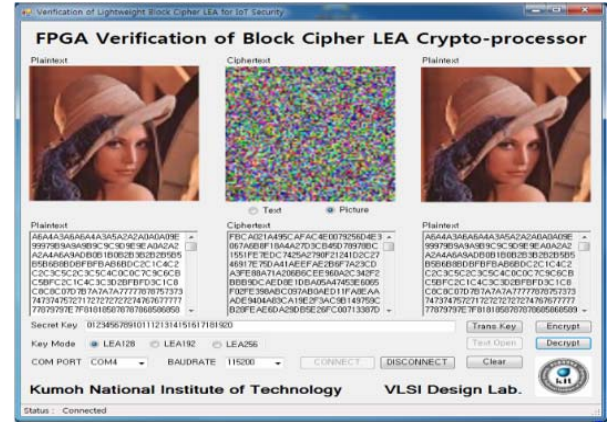
(b) Fig. 9. FPGA verification results of LEA crypto-processor (a) FPGA verification set-up (b) FPGA verification results
