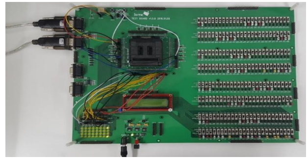
Fig. 3. Test board for verify chip operation
